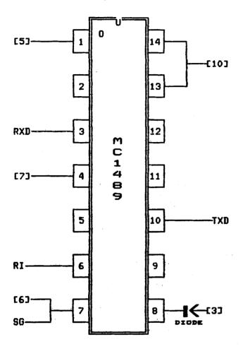
If the cable is never to be used with other peripherals like a 1050 you can omit the diode. If you do use a diode (recommended), ensure that it has low forward voltage. Any germanium diode, and probably, most small signal diodes like the 1N914 will do. Bob Nex and I have built these. The performance is excellent, especially under SpartaDOS.
