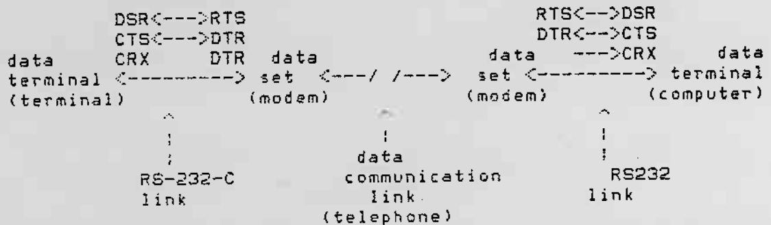
FIGURE 1: COMMUNICATIONS HOOK-UP SHOWING ROLE OF RS-232-C
